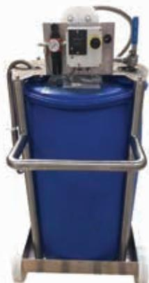
The pneumatically controlled trolley is designed to safely and accurately dose chemical from the onboard 200 litre drum into vessels, tanks, etc. The advantage of this system is that with the drum being an integral part of the trolley it can be filled and emptied without the need for handling of the 200 litre drum. It is easy to use and delivers preset dose volumes from the onboard chemical drum through a delivery hose to a shepherd's crook.
