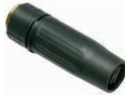
A high-pressure nozzle that allows the adjustment of the spray angle from 0° through to 80° by a simple twist of the nozzle head. The vario nozzle is available in various sizes. The inlet connection is 1/4" female and is suitable for any 1/4" lance.
