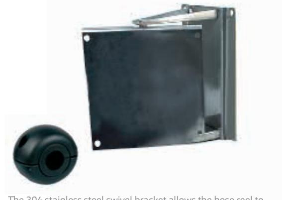
The 304 stainless steel swivel bracket allows the hose reel to pivot left to right through almost 180°, giving greater coverage in a large working area. Pivoting wall brackets also give a more efficient hose pull out & retrieval for the operator, which in turn cuts down the chances of hose stacking should the units be of static mount.
