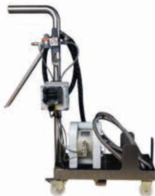
The pneumatically controlled trolley is designed to safely and accurately dose chemical from a 25 litre keg into vessels, tanks, etc. The trolley has a lift up action to allow the safe insertion and removal of the keg. It is easy to use and delivers preset dose volumes, which are set using the onboard batch controller. The chemical is drawn from the onboard chemical keg through a delivery hose to a shepherd's crook.
