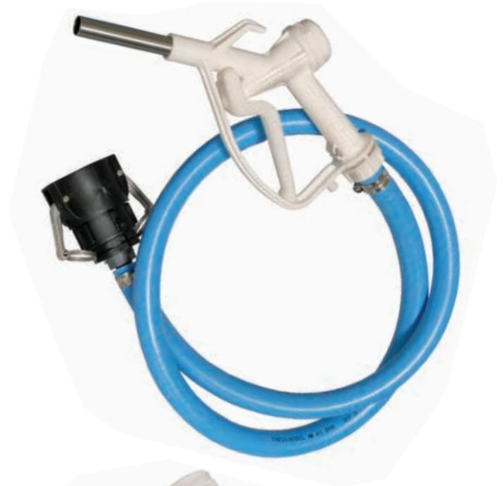
A pair of decant hose assemblies with or without trigger for attaching to a 1 1/2" male camlock on an IBC container, to enable smooth decanting of chemical into smaller containers via a 3/4" hose.
