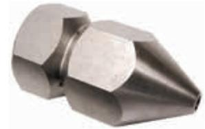
A range of drain nozzles available in various nozzle sizes. The nozzle incorporates one forward and three or four reverse facing jets. The inlet is a 3/8" female.
