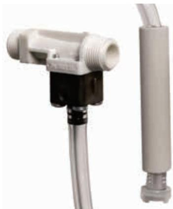
This polypropylene venturi injector provides a safe, controlled and economic method for dilution of chemical on small equipment such as bootwashers. The injector is mounted directly into the pipework and chemical is picked up locally. The strength is controlled by inserting different coloured metering tips.
