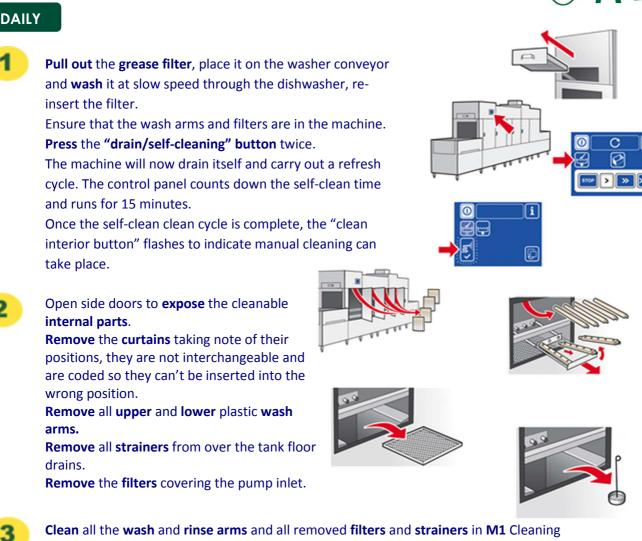
Detergent solution, ensure all nozzles and jets are unblocked.
