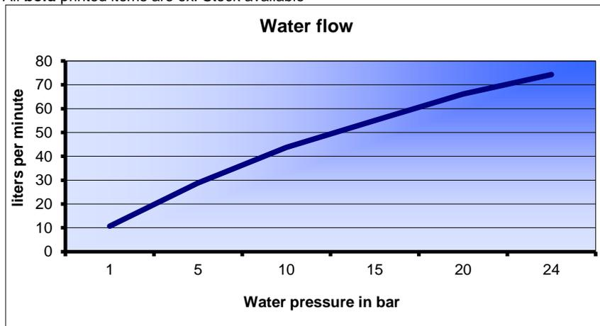
Water flow in l/min with totally pulled trigger
