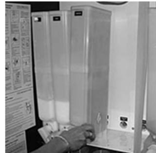
**8** **Remove** the waste water **bucket** from the machine. Empty and **clean**.
