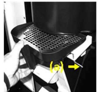
**10** Undo the knurled nuts and **remove** the **cup throat** complete with drain pipe.
