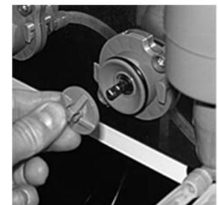
**6** Feed the dispense pipes complete with dispense spouts through the locating holes in the dispense head.
